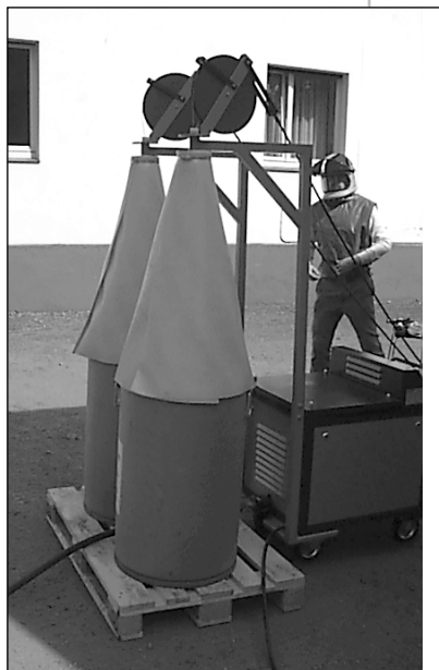
Drum's Feeder for 250 kg Zinc Wire Drums fixed to the Power Source Id.-No. 140142
