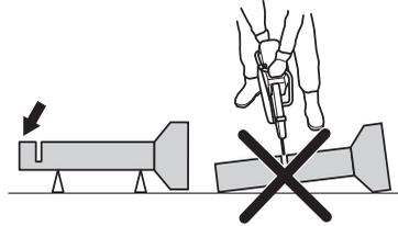
If the pipe is allowed to sag and close the cut, the blade will be pinched in the kick back zone and a severe kick back might develop. If the pipe is properly supported the end of the pipe will move downward, the cut will open and no pinching will occur.
