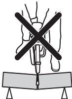
If the blade is pinched or stalled in the kickback zone, the reactive force will push the power cutter up and back towards the user in a rotating motion causing serious or even fatal injury. Be alert for potential movement of the
