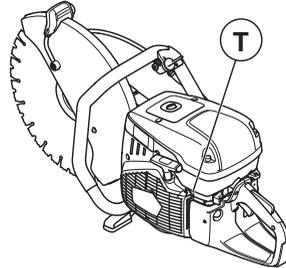
Rec. idle speed: 2700 rpm
