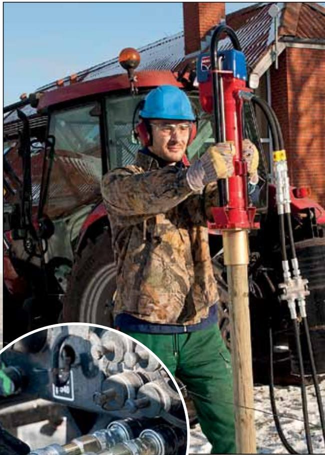
The HYCON Post Driver can be used with onboard hydraulic systems on trucks, tractors, excavators etc.
